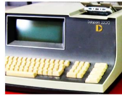
Datapoint 2200 with cassette drive, arguably the world's first Personal Computer. Engineered and manufactured by Datapoint Corporation in San Antonio.
